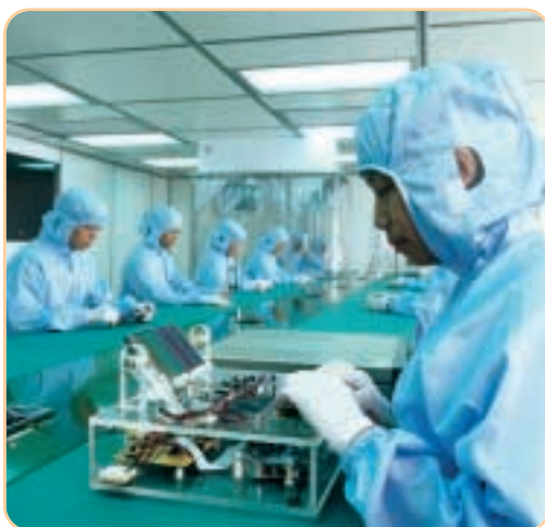
Assembly of LCD Panel in clean zone
